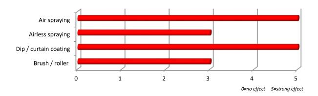
UNIQ®FOAM 170 S is a strong anti-foam and air-release agent especially suitable for use in unsaturated polyesters, baking coatings, epoxies and acrylic/vinyl acetate combinations. The additive furthermore helps to improve the leveling.
